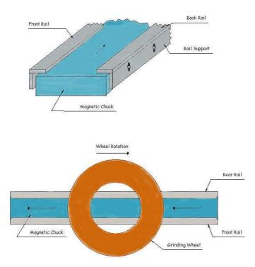
The front rail is necessary for all parts, both magnetic and non-magnetic. It is important to have a space between the guide supports and the magnetic chuck to allow coolant flow and swarf removal. The rear guide rails are important for non-magnetic parts to keep the parts stable in the coolant flow. The rear guide rails also prevent swarf from getting under the abrasive belt. The rails need to be sturdy enough to give stability to the parts.
