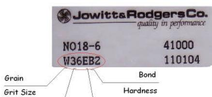
Shown here is a typical product label with our grade marking circled. Our markings are always in the format of Grain, Grit Size, Hardness, Bond. Grain types are identified in the chart below. Grit size is the size of the abrasive grain; smaller numbers for larger grain and larger numbers for smaller grain. Our bonds all start with 'B', signifying resin bonds.
