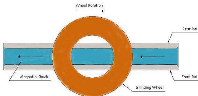
The front rail is necessary for all parts, both magnetic and non-magnetic. It is important to have a space between the guide supports and the magnetic chuck to allow coolant flow and swarf removal. The rear guide rails are important for non-magnetic parts to keep the parts stable in the coolant flow. The rear guide rails also prevent swarf from getting under the abrasive belt. The rails need to be sturdy enough to give stability to the parts.
